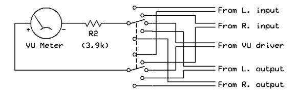
And, -because the GSSL uses differentially-balanced outputs Using a 2-pole 2-way switch, the meter can also cunningly be switched between GR and a sum of both outputs like so:
