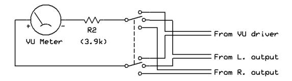
Using a 2-pole 5-way switch, the meter can be switched between input-left, input-right, GR, output-left and output-right like so:
