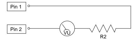
Bear in mind that a true VU meter pays no attention to polarity, so it can be connected either way around with no difference. Also, it doesn't matter whether the resistor goes before or after the VU meter. –Basically, so long as they're connected together in series as shown, everything should work correctly.
