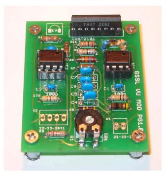
Here is a picture of the assembled board. Among other things, it shows how the four 100nF capacitors are all grouped together, while the three 100pF capacitors are nearer to the two 5532 IC's. The VCA in this instance is a 2150 series (though it could also be a 2180 series).
