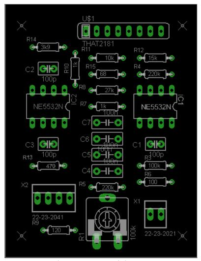
There are two connectors, X1 and X2. X1 is very simple to connect; it only has two pins, connect one pin to one end of the VU meter/R2 combination, and the other pin to the other end, as shown:
